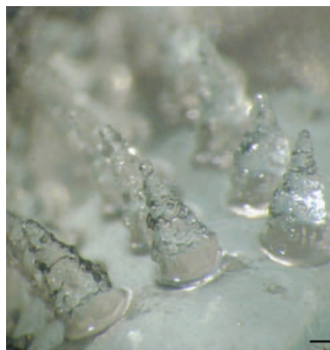
Figure 14 Representative light microscopy image showing an intact hydrogel MN array (containing 5% NaHCO 3 ) following removal from neonatal porcine skin after a period of 24 h. Scale bar represents a length of 300 \mu m. [Color figure can be viewed in the online issue, which is available at wileyonlinelibrary.com .]
